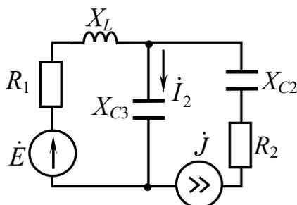
$$\begin{aligned}X_L &= X_{C2} = 10 \text{ Ом} \\R_1 &= R_2 = 10 \text{ Ом} \\X_{C3} &= 20 \text{ Ом} \\E &= 10 \text{ В} \\J &= 2 \text{ А}\end{aligned}$$
